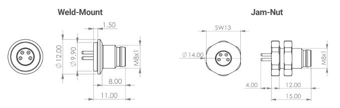
For the best performance and lowest leak-rates we recommend the weld mount installation if possible.
